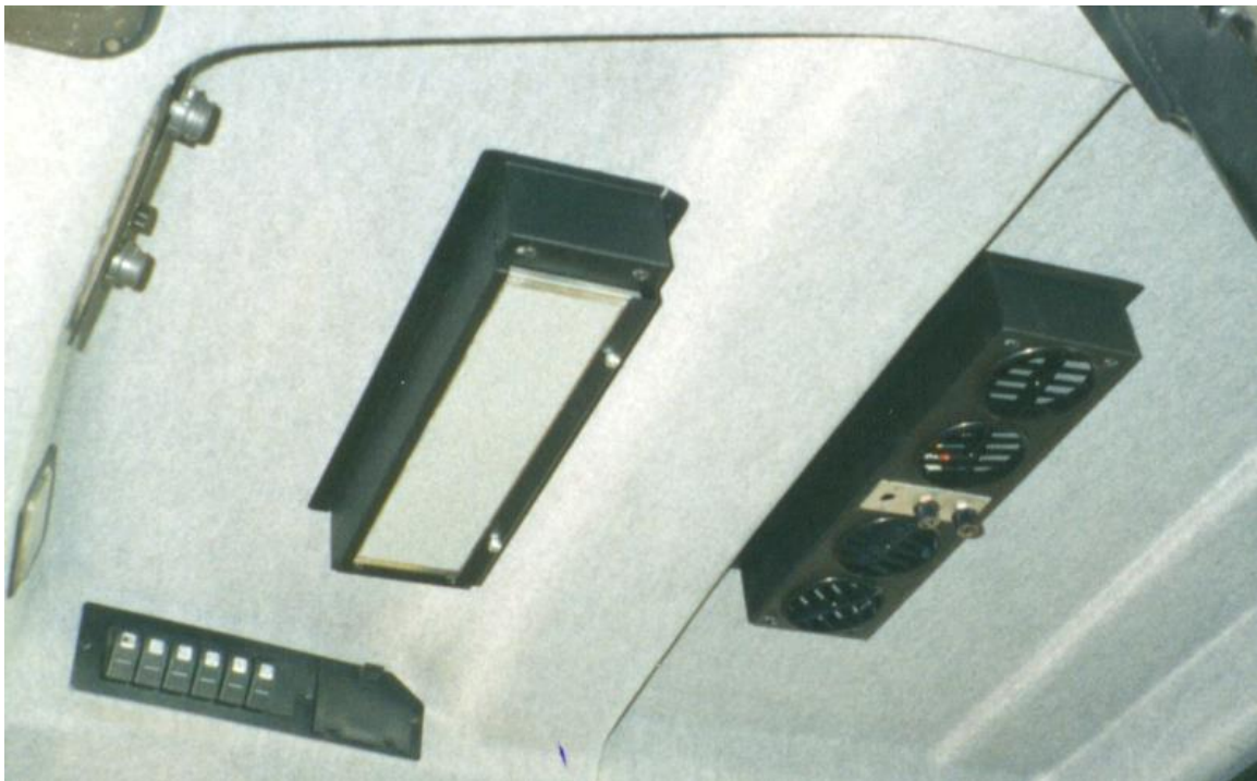
Air delivery, filter and controls in place.
