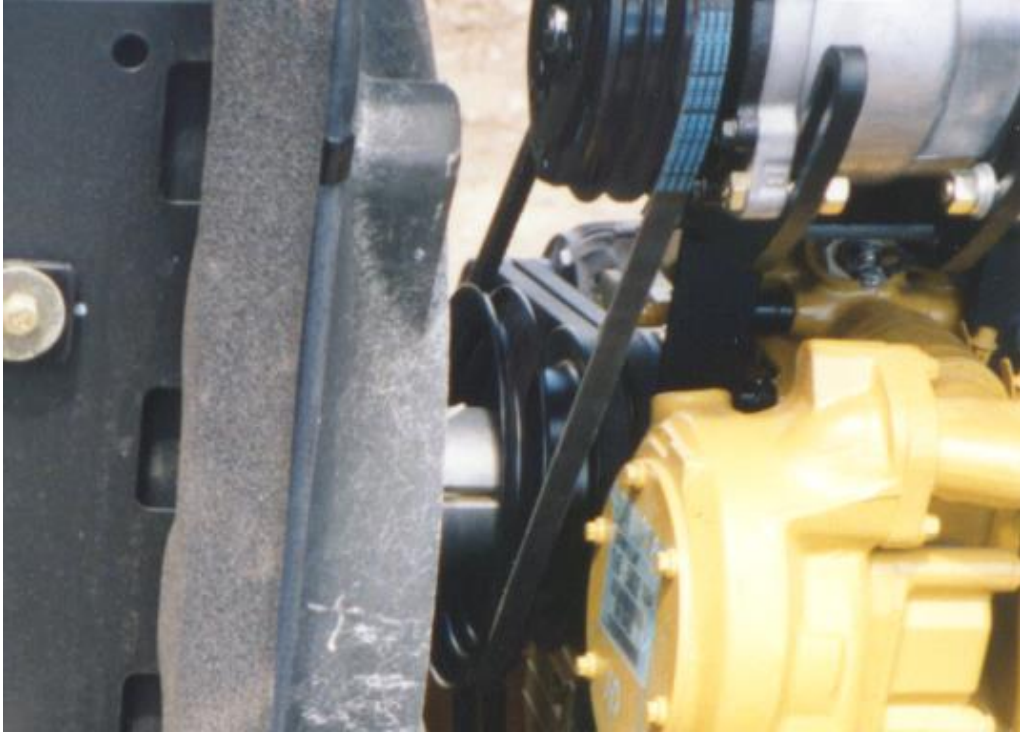
View showing drive pulley and V-belt to compressor.
