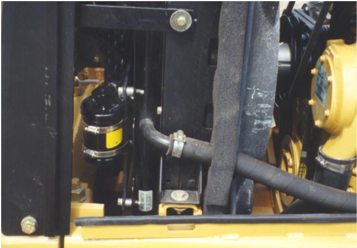
Condenser in place with drier and spacers shown (older version).
